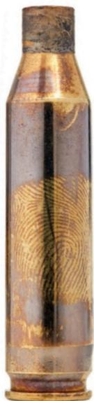
Vacuum Metal Deposition (VMD) is known to develop high quality fingerprints on difficult substrates. West Technology Forensics recently undertook a two (2) month research study to test VMD's capabilities to develop fingerprints on fired ammunition—a notoriously challenging exhibit from which to recover fingerprints.
