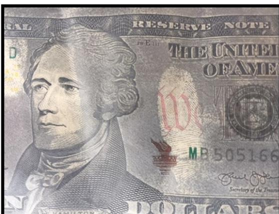
Vacuum Metal Deposition (VMD) has developed latent fingerprints on evidence that is over twenty (20) years old. The technique has also provided remarkable results on exhibits that have been submerged in water or buried underground.
